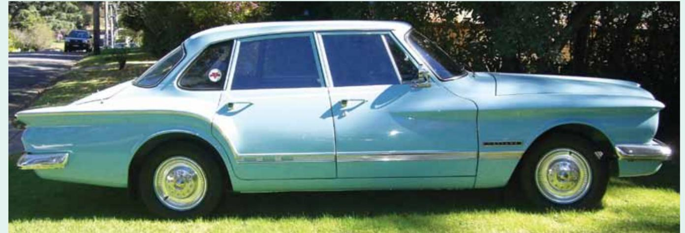
**The "S" Series** is very similar in appearance to the "R" Series with outward cosmetic changes distinguishing it from its predecessor. Removed was the fake wheel mold on the boot lid, the "cat's eyes" tail lights were changed to a more conventional tail light assembly, a different grille installed and changes to much of the chrome work. The floor mounted manual shift was moved to the steering column plus several other mechanical alterations were included.
